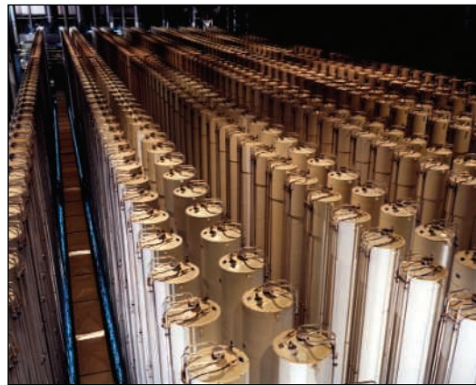
Spin control. Most countries have adopted nonlaser methods for enriching uranium, such as spinning it in gas centrifuges like these.
